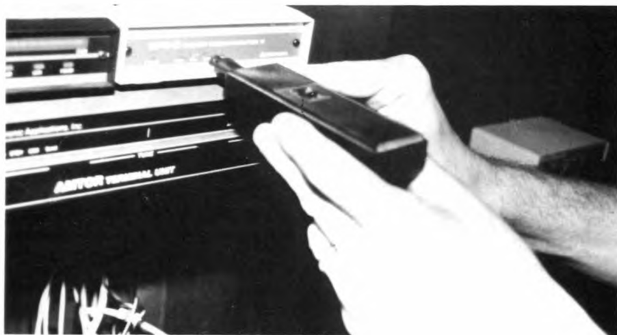
Fig 3—The Squawker being used to check LEDs on a KPC-2 packet modem.
