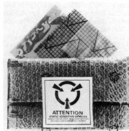
Fig 3—Static-dissipative circuit-board packaging makes use of a variety of materials. The padded circuit-board envelope (foreground) is constructed with a heavy, carbon-impregnated vinyl lining that is covered by a protective layer of air-filled cells. The three circuit-board jackets (background), while providing minimal padding, are also constructed of static-dissipative materials. The highly reflective metallized jacket (top left) provides a complete electrostatic shield, at the expense of poor circuit-board visibility. The jacket with the dark grid pattern (top center) formed by conductive traces impregnated into the otherwise nonconductive clear plastic, provides less-complete electrostatic shielding, but allows easy inspection of the enclosed circuit board. The nearly transparent jacket (top right), provides less electrostatic shielding than the other designs, but also minimally impairs visual inspection.
