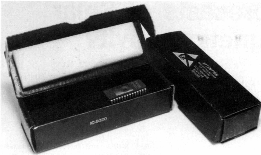
Fig 2—The lightweight and sturdy containers shown here are designed for mailing and storage of static-sensitive components.
