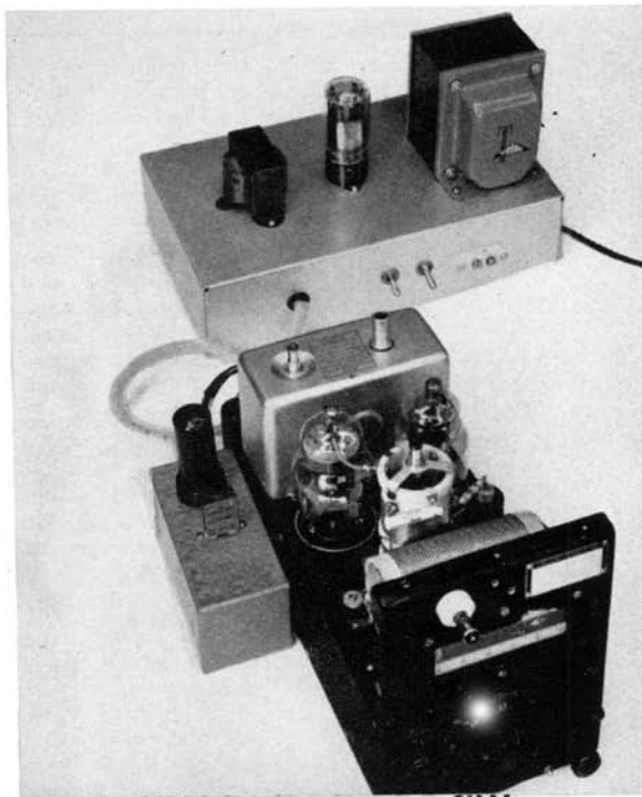
Fig. 6-90—The complete Novice setup, in this case using the 80-meter (BC-457) transmitter. Note the key jack at the lower-left corner of the transmitter panel. The crystal oscillator is connected to the transmitter oscillator-tube socket with a short length of cable terminating in an octal plug. A small notch should be cut in the transmitter cover to provide clearance for the cable when the cover is installed.
