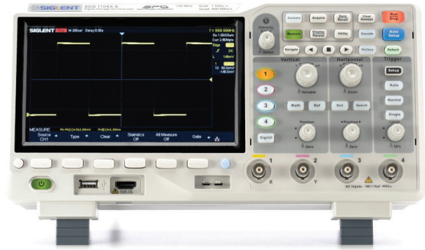
Figure 7 — The Siglent Technologies SDS1104X-E. The LAN and USB connectors on the lower left are used to input programs, control the unit, update the firmware, and save screen data.
