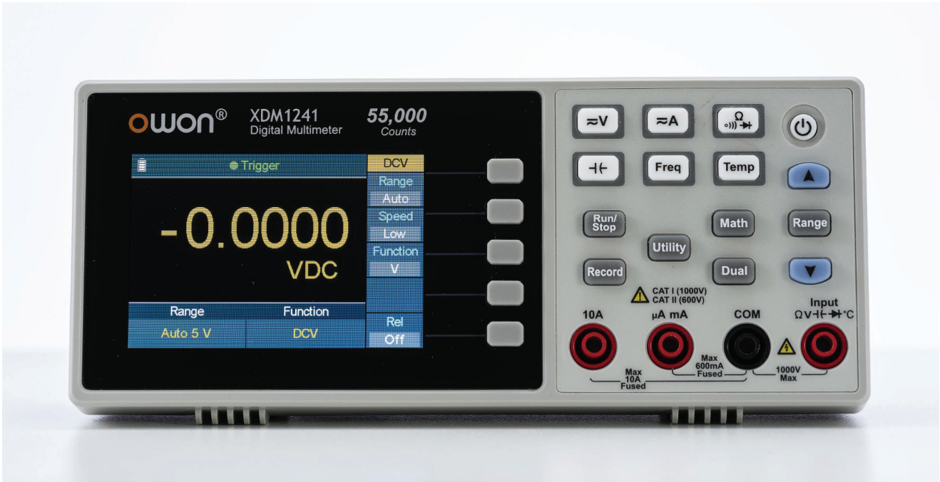
Figure 3 — A digital meter front panel. You can see the LCD panel (left), the soft switches (middle), and the mechanical switches (right).
