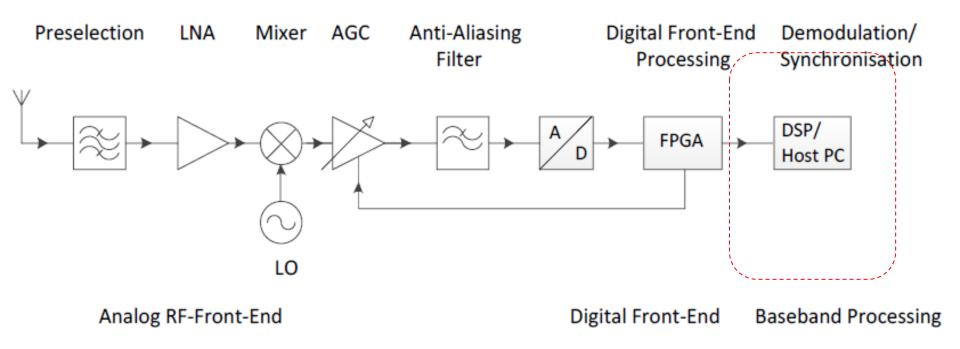
The baseband processing takes over the base band filtering, AGC, demodulation, and the signal regeneration..
