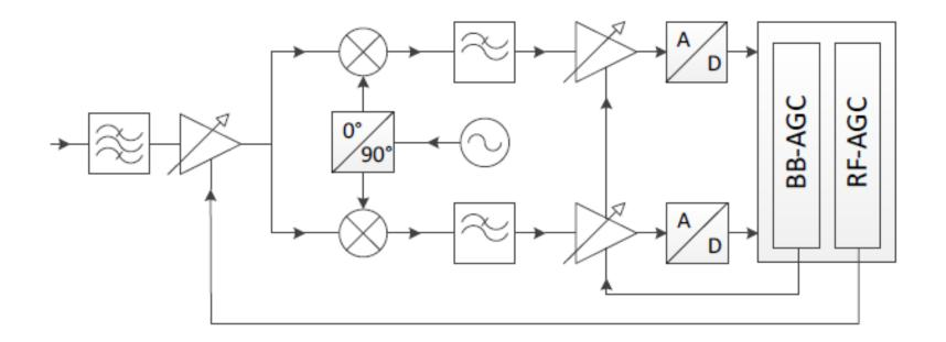
The broadband AGC serves to protect the AD converter from overvoltages. The RF-AGC can be used to set the receiver sensitivity just below the external noise.
