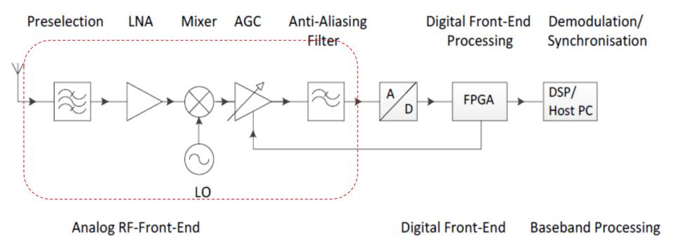
The analog front end is downconverting the RF signals into an IF range <200MHz
