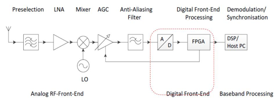
The digital front end consists of an Analog to Digital converter and a digital down- converter to reduce the sample rate down to the bandwidth needed by the application. Sampling rate of AD converters are rising up to 250Msps with resolutions of 14 or 16 bits.
