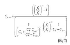
The holder capacitance of the crystal will be the value of  $C_h$  that makes  $C_{m10}$  equal to  $C_{m20}$ , which will then be the motional capacitance  $C_m$ . I don't have an analytical solution for determining  $C_h$  so I solve it numerically. For AT-cut crystals in standard or low profile HC49 packages,  $C_h$  will be within the range 1.5 to 6 pF. The microprocessor controller measures the three frequencies and then steps
