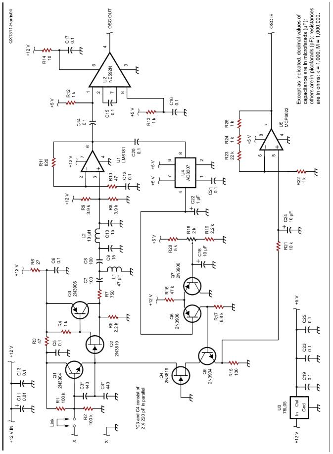
Figure 4 — This schematic shows the amplitude controlled Colpitts oscillator circuit used in the author's test system.
