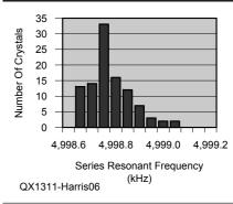
Figure. 6 — This graph shows the spread of series resonant frequencies,  $f_{s}$ , for the same 100 crystals.
