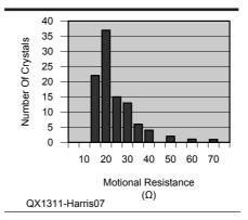
Figure. 7 — This graph shows the spread of motional resistance, *R*<sub>m</sub>, for the batch of 100 crystals.
