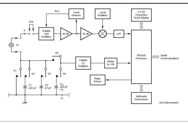
Figure 3 — The schematic/block diagram hybrid of the author's crystal measurement unit.
