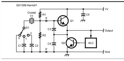
Figure 1 — This schematic is a basic crystal test circuit.
