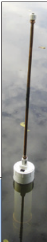
Figure 4 — The buoy is ballasted to keep the GPS antenna above the water line.
