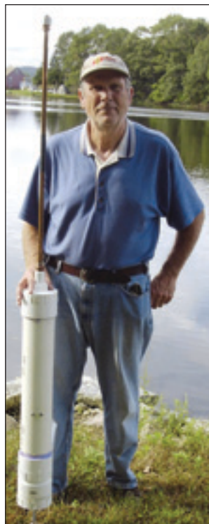
Figure 3 — Buoy body constructed out of common PVC plumbing fixtures available in home improvement retail stores.
