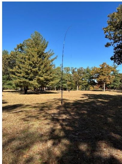
“Sotabeams dipole with Spiderbeam fiberglass telescoping mast on 40 meters”
