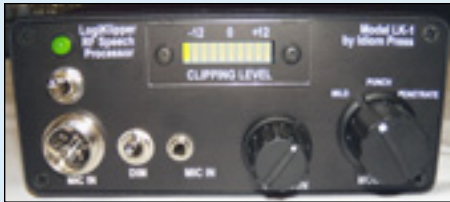
The Idiom Press LK-1 RR speech processor increases effective RF power output of SSB transceivers.
