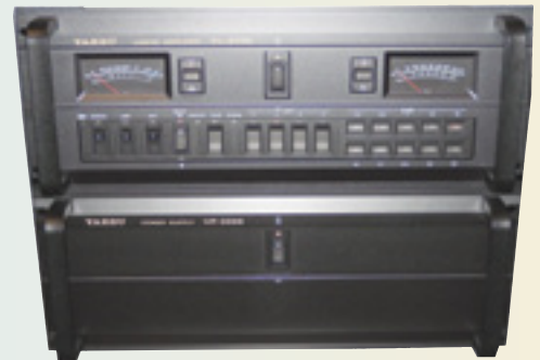
Yaesu's VL-2000 HF and 6 meter legal limit linear amplifier.
