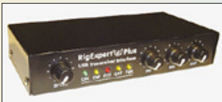
RigExpert Plus multimode transceiver to computer interface with USB connectivity.
