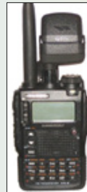
Yaesu VX-8DR V/UHF four band handheld transceiver with built-in GPS and APRS capability.
