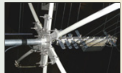
DX Engineering balanced multipoint feed for Hexx beam antennas.
