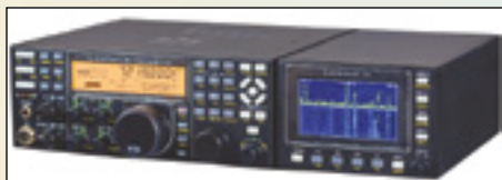
Elecraft stand-alone P3 panoramic receiver (panadapter) displays signals received on their K3 HF and 6 meter transceiver.
