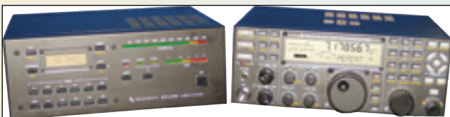
The new compact, self contained, Elecraft KPA-500, 500 W HF and 6 meter amplifier shown next to the K3 transceiver.
