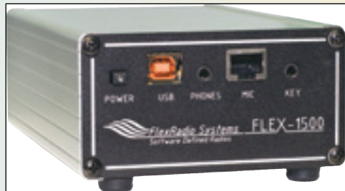
The FlexRadio FLEX-1500 entry level SDR HF and 6 meter transceiver.
