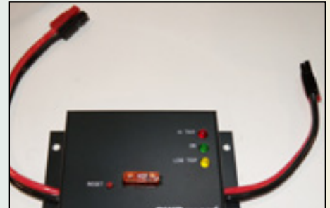
West Mountain Radio PWRguard protects radio equipment from high voltage spikes on a 12 V dc line.
