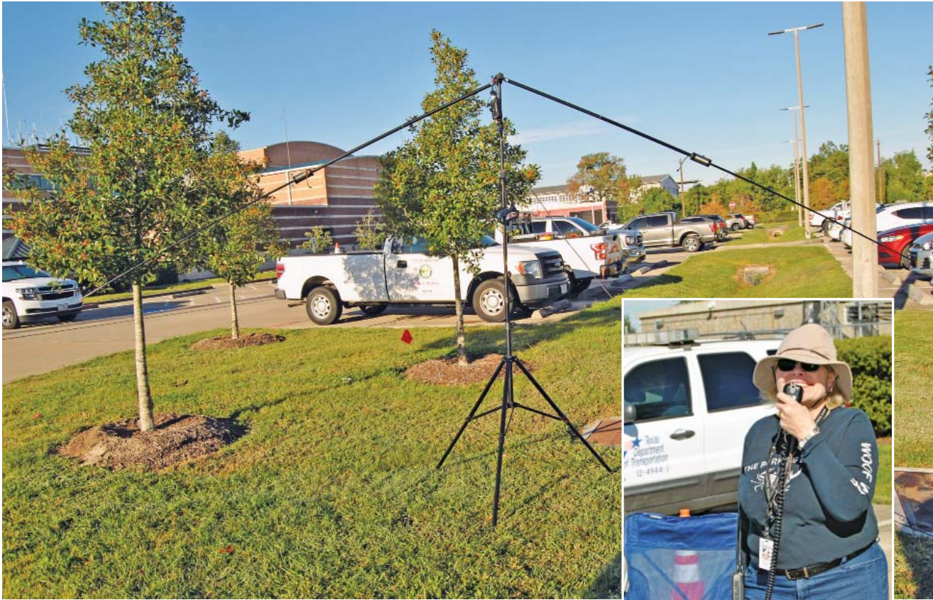
Peter Aronstam, KW5PA, set up an inverted V Buddipole antenna for NVIS.
